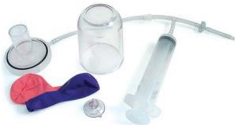
Students can now safely produce a vacuum in a small bell jar right at their lab stations. By reducing the pressure in the microscale bell jar, they can expand a balloon, boil warm water, and even transfer liquids from one pipet to another. They can watch a marshmallow or shaving cream increase in volume as the pressure is reduced and learn about how extremely low pressure affects the world around them.
