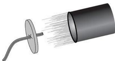
These amazing piezoelectric devices generate a few thousand volt sparks at the touch of a button. No batteries required. The discharge is created when a small hammer inside the device strikes a quartz crystal. It can be used as a safety lesson to demonstrate the flammability of alcohol or perfume. Igniting two drops of alcohol in a film canister will cause the canister to fly more than 20 feet into the air! Kit includes piezo igniter, instructions, film canister, wire and connector.
