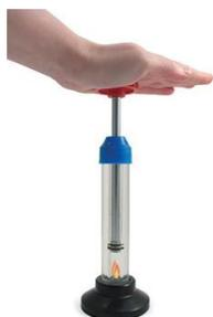
When the piston in the transparent cylinder is rapidly depressed using a quick, firm stroke over dry cotton or paper tissue fibers, ignition occurs. The compression of the air causes the temperature of the gas to rise rapidly, igniting the material at the base of the cylinder resulting in a bright flash. This is one of the most impressive demonstrations of the heat produced when a gas is rapidly compressed and is the principle behind how a diesel engine functions.
